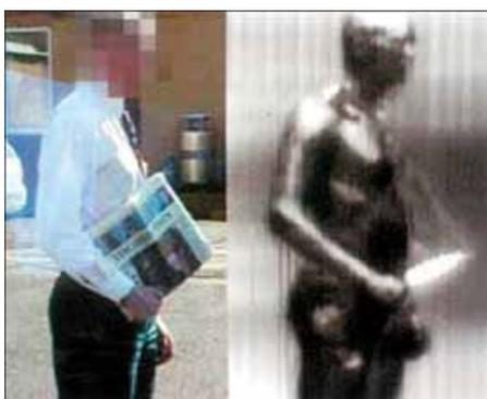
Terahertz radiation can penetrate a wide range of non-conducting materials but can be reflected by dense materials and metals leading to the first application in security screening – see picture below from [Terahertz Science and Technology Network](#). There is likely to be increased research in this area developing further applications.
