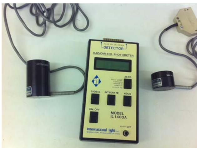
Figure 6. Solid State Radiometer with detectors
